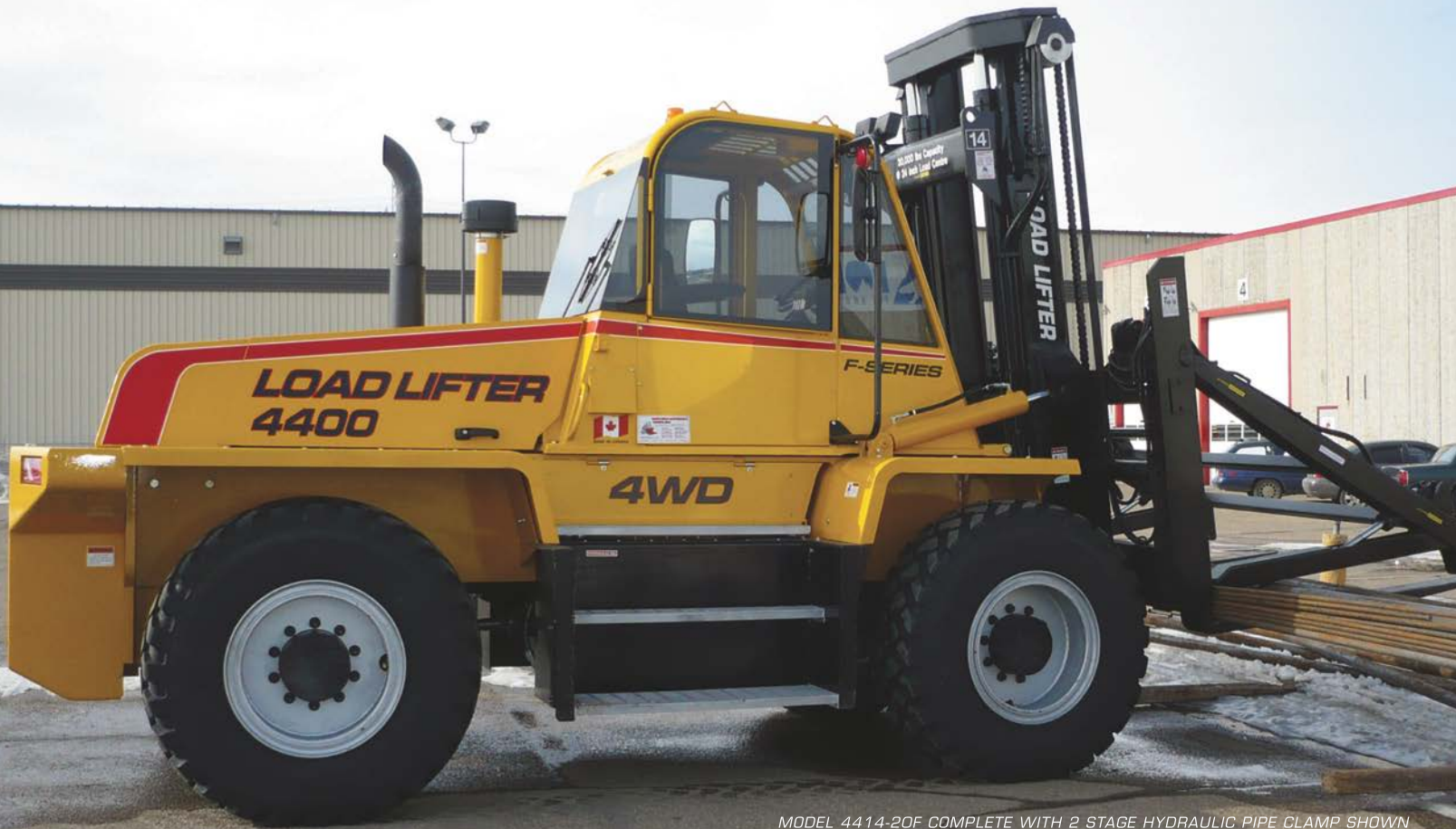
MODEL 4414-20F COMPLETE WITH 2 STAGE HYDRAULIC PIPE CLAMP SHOWN
