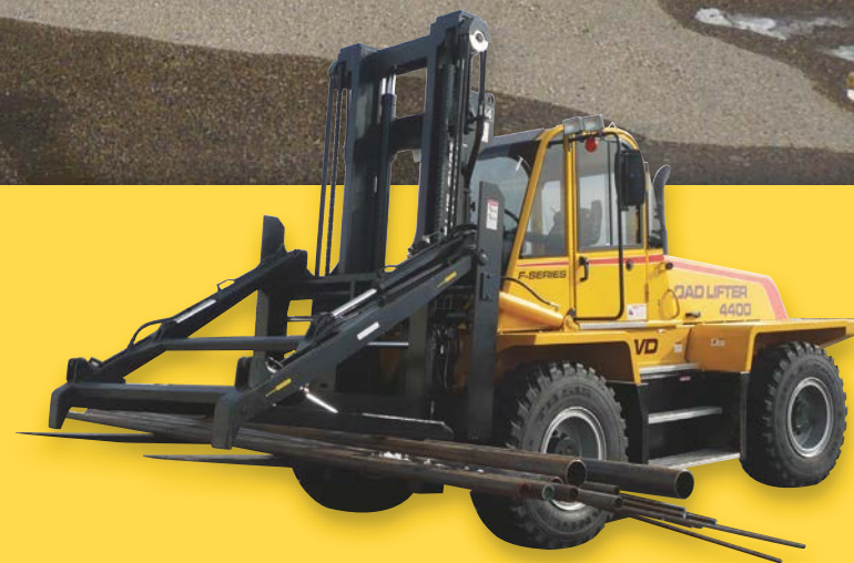
MODEL 4414-20F COMPLETE WITH 2 STAGE HYDRAULIC PIPE CLAMP SHOWN
